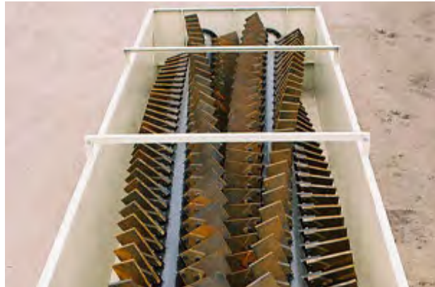
SPIRAL PADDLES FOR CONTINUOUS AGITATION
