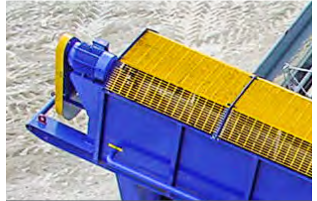
PERSONAL SAFETY COVERS AND GUARDING
