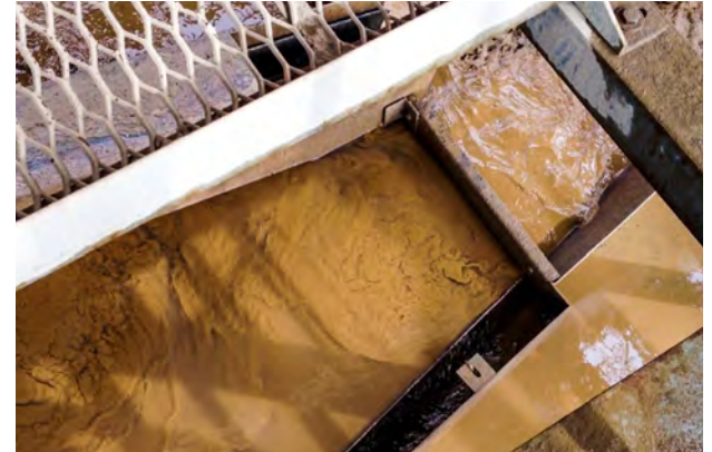
LOAD ZONE Baffle SETTLES FINES
