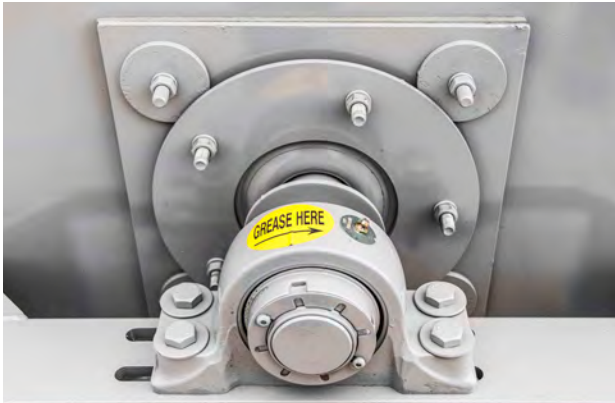
SLINGER PROTECTS LOWER BEARING
