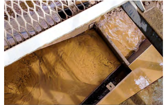
LOAD ZONE BAFFLE SETTLES FINES
