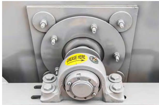
SLINGER PLATE PROTECTS LOWER BEARING
